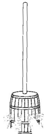
Figure 2.6: Pascal's rain barrel. From Martin and Conner, Basic Physics , 8th ed., published by Whitcombe & Tombs Pty. Ltd., Melbourne, Australia, 1962, with permission.
